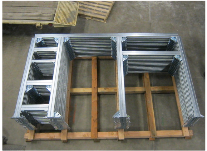
Pre-assembled Pipe Racks
